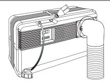
Insert the tip of the bottle into the connection nozzle on the device and slowly squeeze the entire contents into the opening.
