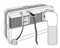
2. Disconnect the exhaust hose from the device.
