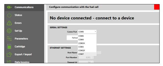
Once the proper port is selected you can complete the connection by clicking on the Connect button (Connect COM7 in the example below).
