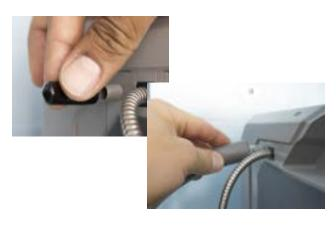
15. If you're utilizing any communications with your EFOY Fuel Cell, you can connect the cable to the LAN port seen below.
