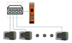
Note: The CC2 communicates with EFOY devices using the ModbusTCP protocol over Ethernet connections. Each device in the cluster, including EFOYs and the CC2 itself, must be in the same IP subnet. EFOYs are configured to use dynamic addresses by default. The CC2 will automatically detect if a DHCP server is present;
