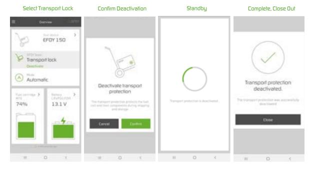
19c. Put the EFOY into 'Automatic' operating mode. The EFOY will sense when the voltage in the batteries is drawn down to the switch-on voltage threshold and automatically switch on to begin a charging cycle whenever required.
