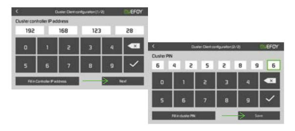
Note: The connection may be blocked if the DHCP Client is currently enabled. To rectify this, you can return to the 'EFOY Fuel Cell' menu and go into the 'Ethernet Configuration' menu. There you will see a toggle switch called DHCP Client, and if it's currently green, and enabled, select it to disable it.
