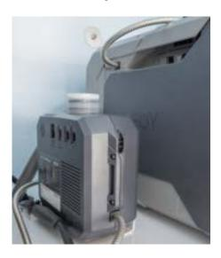
6. Secure the EFOY fuel cell into place by running the strap though the mounting brackets.
