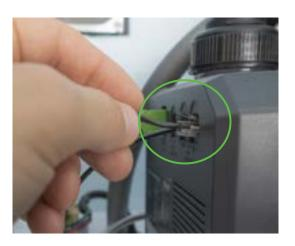
16. Connect the EFOY Fuel Cell to the system batteries with the charge/sense wiring harness. The large leads are the charging lines, the small leads are the voltage sense lines. They connect to the port on the EFOY as shown below.
