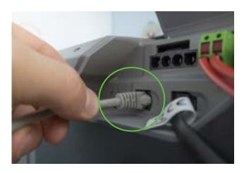
14. Connect the OP3 Operating Panel (touchscreen display) cable to the SFC Bus port on the <u>Fuel Manager.</u>
