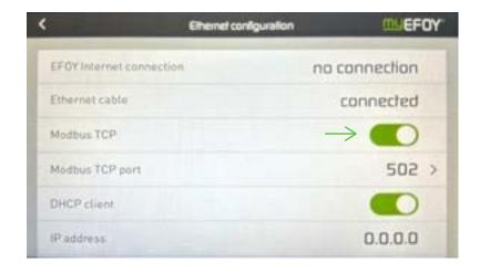
Note: The CC2 will put every EFOY that is in the cluster in the Automatic operation mode using the Modbus protocol. If the user sets the Manual or Off operation mode, either through the display or serial connection, this mode will be overwritten by the CC2 and forced to the Automatic mode.
