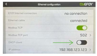
4. Then, you can select 'IP address' and continue to manually input the desired IP address and hit Confirm. This will conclude the process.
