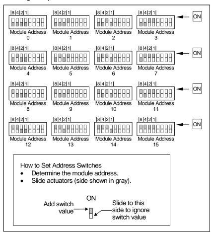
Figure 3: 5405 Digital Input Module Address Switches
