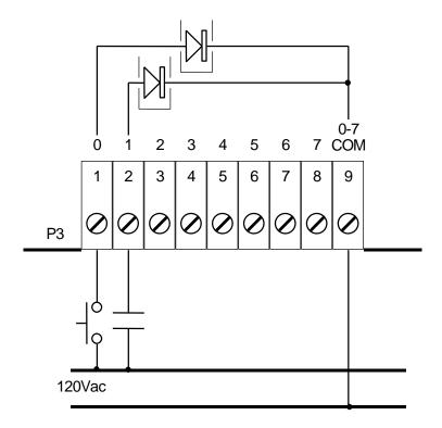
Figure 1: AC Input Wiring Example
