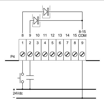
Figure 2: DC Input Wiring Example
