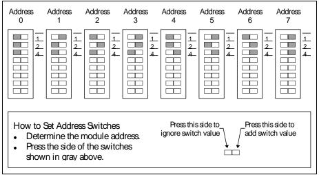
Figure 2: Model 5403 Module Address Switches
