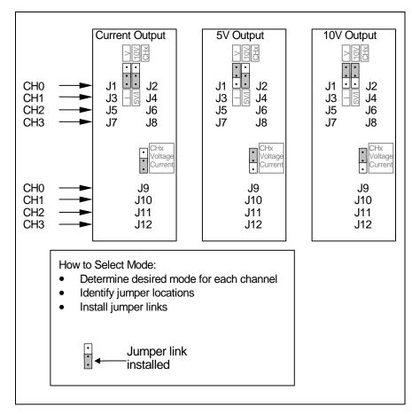
Figure 3: 5304 Current/ Voltage Mode Selection
