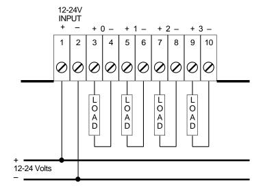
Figure 1: 5304 Typical Field Wiring
