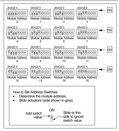
Figure 2: 5304 Analog Output Module Address Switches
