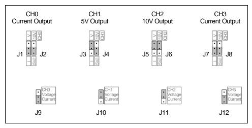
Figure 4: 5304 Mixed Configuration Example
