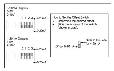
Figure 5: 5304 Output Offset Switch
