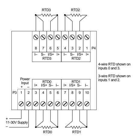
Figure 1: Typical 5505 RTD Field Wiring
