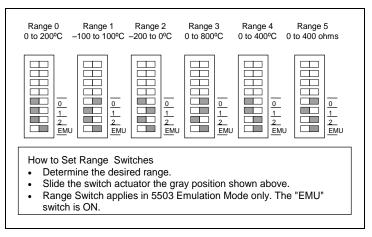
Figure 3: 5503 Emulation Module RTD Range Switches
