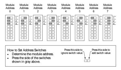
Figure 2: 5503 Analog Input Module Address Switches
