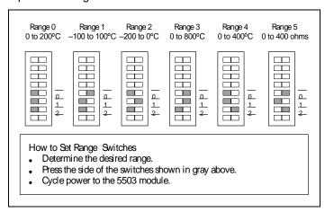
Figure 3: 5503 Module RTD Range Switches
