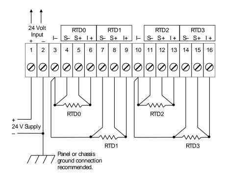
Figure 1: Typical 5503 RTD Field Wiring
