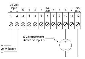
Figure 2: 5501 Typical 5 Volt Field Wiring
