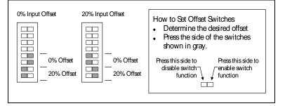
Figure 4: 5501 Input Offset Switches
