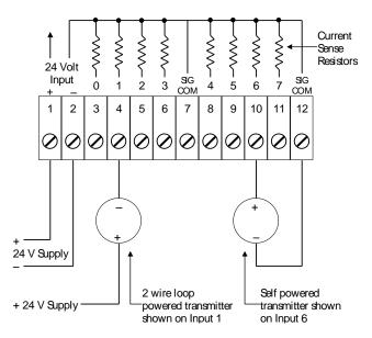
Figure 1: 5501 Typical 20mA Field Wiring
