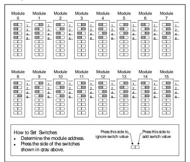
Figure 3: 5501 Analog Input Module Address Switches
