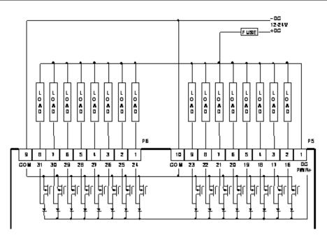
Figure 2: Typical Field Wiring Digital Outputs 16-31
