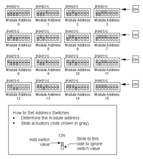
Figure 3: 5411 Digital Output Module Address Switches
