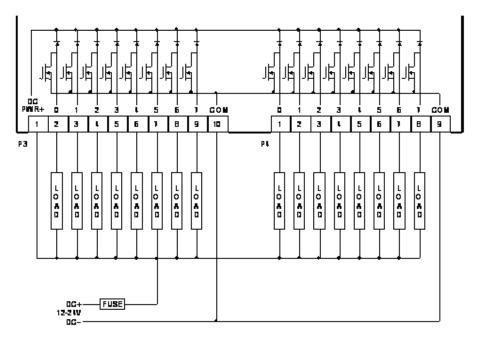
Figure 1: Typical Field Wiring Digital Outputs 0-15
