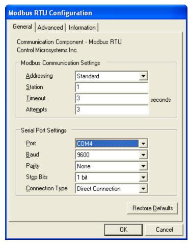
The factory default serial settings for the 5913 are 9600 baud, 8 data bits, no parity and 1 stop bit. COM4 is the virtual serial port created during the installation of the 5914 USB software driver.
