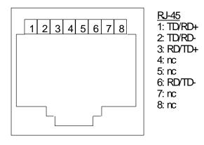
Figure 2: 5905 Ethernet RJ-45 Connection
