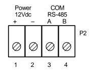
Figure 5: RS-485 Connections
