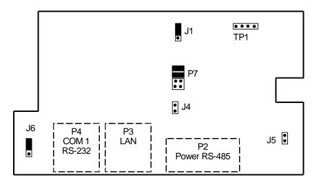
Figure 8: Jumper Layout
