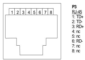
used. See *Figure 6: 5906 Ethernet Gateway RJ-45 Connector* for pin connections.
