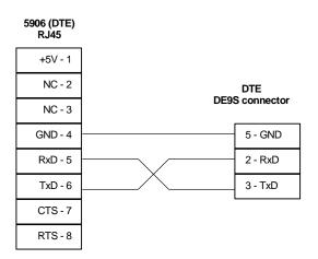
Figure 4: RS-232 Wiring - 5906 (DTE) to DTE
