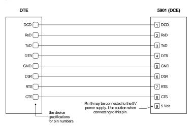
Figure 3: RS-232 Wiring - 5901 (DCE) to DTE
