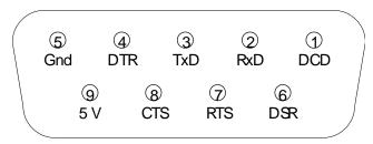
Figure 2: RS-232 Port Connector (DCE)
