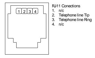
Figure 4: 5901 Modem RJ-11 Connection, P6
