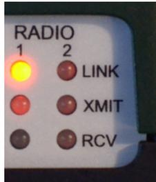
The **LINK** LED shows radio power and link state.
